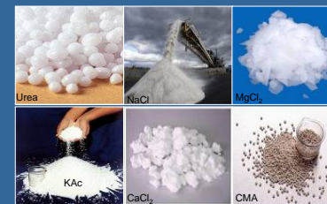
Figure 4. Six chemicals commonly used for chemical deicing and anti-icing procedures in North America.
